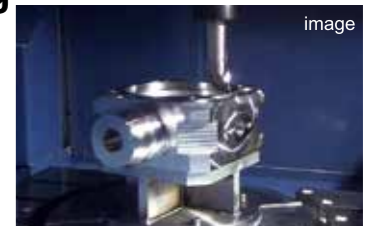
* Synchro Tip (Orbit machining + C-axis rotation)
